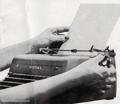
A. Pull forward Automatic Paper Lock and drop paper behind cylinder onto Royal's single wide rear feed roll which acts as a straight edge, guiding the left edge of paper against paper guide.
